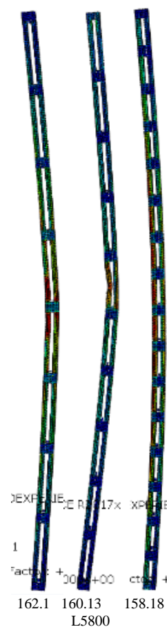
(a) Non-linear FE analysis deformed shapes for series B40 with overall slenderness ratio( \lambda ) from (66.08to 162.1)
